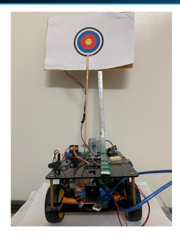
We found that our Autonomous Target Robot was most successful on flat, hard surfaces such as concrete or asphalt. We also found that the further away we got form buildings, the more accurate our GPS coordinates were. This helped us to determine the optimal conditions for operating our vehicle - a long-distance target range with flat, solid ground. Our vehicle was also able to operate in conditions of wet ground and in grass with more limited mobility.
